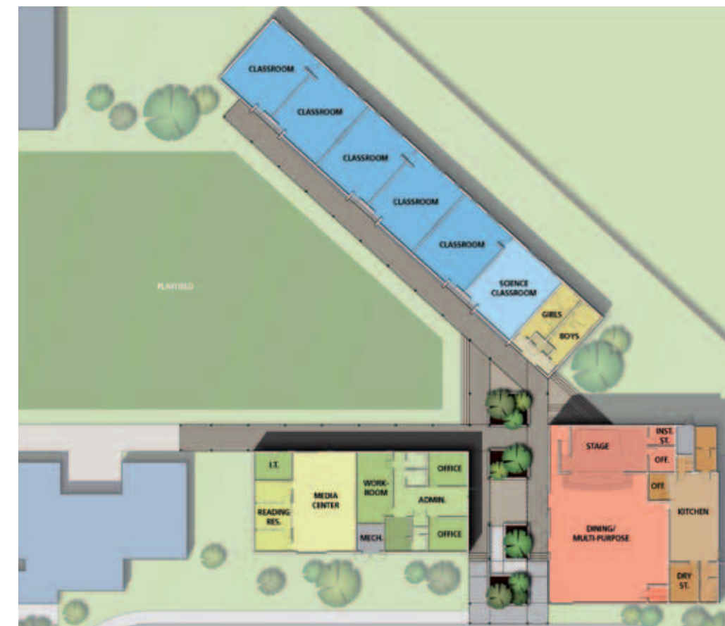
Wimauma Academy’s middle-school expansion will add six classrooms, a cafeteria and a media center at the eastern end of the current campus.
